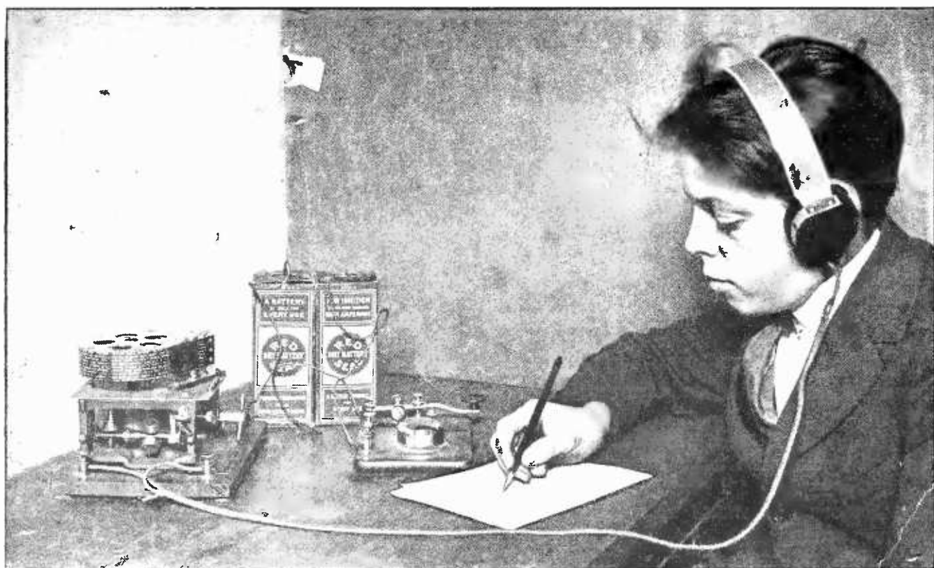
AN AUTOMATIC SENDER IS A GREAT HELP TO THE WOULD-BE TELEGRAPHER
